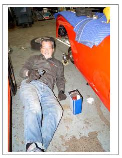
brakes and windscreen. After installing the new clutch/brake master cylinder the team flushed the hydraulic system with denatured alcohol. Brake and clutch hoses were installed and the plan for a future work day, is to fill the master cylinder with brake fluid, bleed the system, fix any leaks and go from there..
