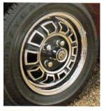
The V8 model had this style of composite wheel, with a cast alloy centre and a chrome-plated steel rim. This wheel was also found on the 1975 GT 'Jubilee' model, on which the bright parts were painted gold.
