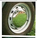
The 15in disc wheels fitted to the MGC were quite different from those on the MGB, with elongated instead of circular holes, and the characteristic beveled edge to the hubcap.
