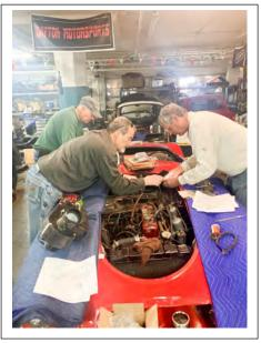
windscreen. The new clutch/brake master cylinder was installed by Bill Hunter, Dave Gribler and Ron Ramer. The plan is to flush the hydraulic system with denatured alcohol, then refill the system with Dot 5, silicone brake fluid.
