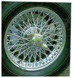
Alternatively the MGC could be fitted with 72-spoke wire wheels, either painted or chrome plated, as seen here. The knock-ons were fitted only during the first year of MGC production.
