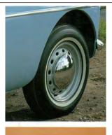
Fitted as standard equipment on MGB cars from 1962 to 1969, the painted disc wheel was painted in a silver colour -probably the BMC colour 'Aluminium' – and fitted with this simple hubcap design. The narrow-band whitewall tyres seen on this car are probably not the correct type for a pre-1963 car.
