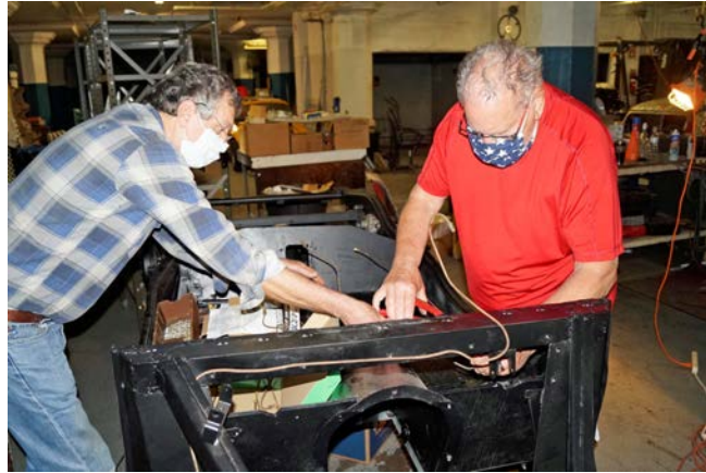
Dave Gribler and Ron Ramer installing brake lines
