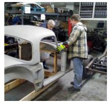
The frame and suspension parts are back in the museum after having been blasted, primed and painted by Dayton Metal Prep, Inc. We have begun putting parts back onto the frame. Our intention is to create a running chassis prior to setting the body on the frame. Work on prepping the body parts is continuing as well. Once this is complete to our satisfaction, we will have the body shop come and
