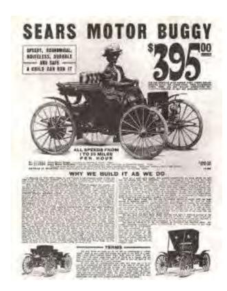
The cars were manufactured by the Lincoln Motor Car Works and powered by a two-cylinder engine with 10 hp that gave them a top speed of just 25 mph.
