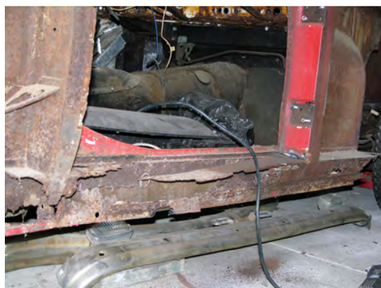
Rust damage to the right rocker. What a mess! Left side was just as bad.
