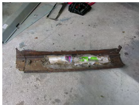
"Professional" rocker repair with cardboard, unsaturated fiberglass, and Bondo! No new metal here.
