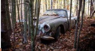
engine and paint job it appears to have picked up prior to its trip east. Its 3.7-liter inline six was rated at 240 hp when new, and the car features a 4-speed transmission with Laycock Overdrive, disc brakes and "knock-off" wire wheels.
