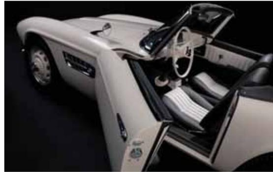
The 507 was completely disassembled, and the paint removed with acid and alkaline baths. Many replacement parts were recreated using a mix of old and new manufacturing methods, with extras made for other 507s in need. It’s no surprise that the Chevy V8 was replaced with a correct BMW 3.2-liter V8.
