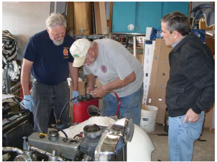
Jim Pesta (L) instructs Bob Hanseman (C) on how to read the two pressure gauges to determine the amount of air leakage. Steve Veris watches intently.
