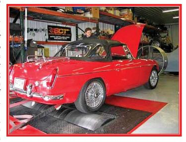
dynamometer measured horse power versus engine speed, the air to fuel ratio versus engine speed and the torque versus engine speed. The maximum torque out of three runs came in at 127 foot pounds; the maximum power on one of the runs was about 95 horse power.
