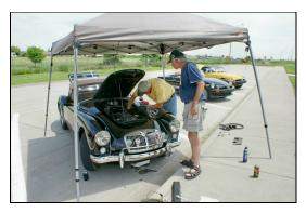
While Ryan was off acquiring a compression tester, a wire brush, additional sets of spark plugs for spares, and a few other needed items, the party/work tent was extracted from the Looft's trailer and setup, so that if a head gasket replacement was needed, it could be at least accomplished in the relative shade of the tent. Once the compression was tested, no pressure was measured in cylinder 2 or 3, indicating the gasket was blown between cylinder 2 and 3 and the teardown began.
